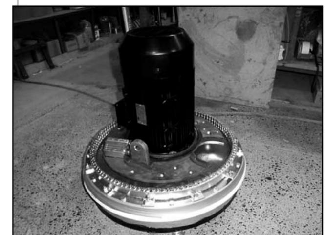
Lift off machine cover to reveal chain ring and planetary seal.
