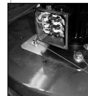
Remove cover off motor terminal box.
