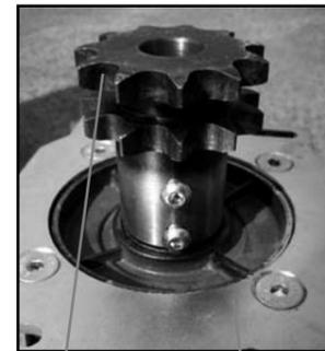
1. Planetary drive sprocket
